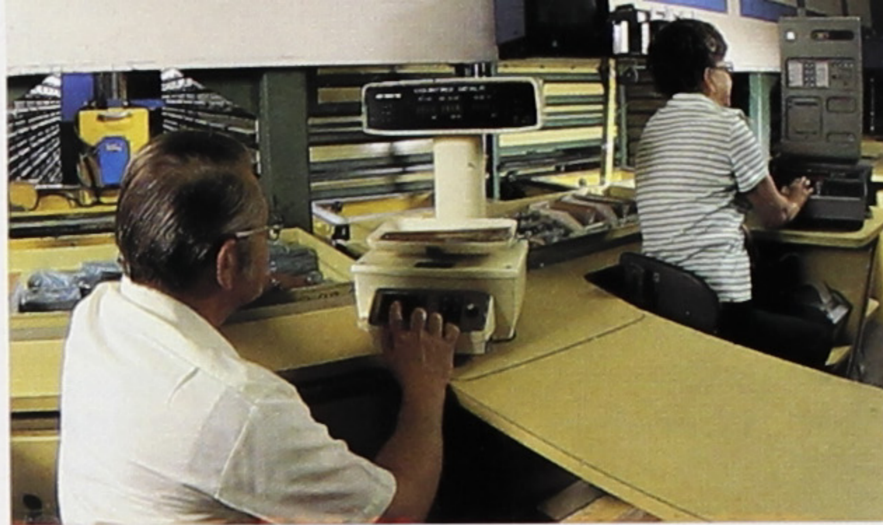
Litton UHS's Automove™ "miniload" system (left) is essentially an automatic warehouse for small items. It improves inventory controls and space utilization, generating cost savings.
