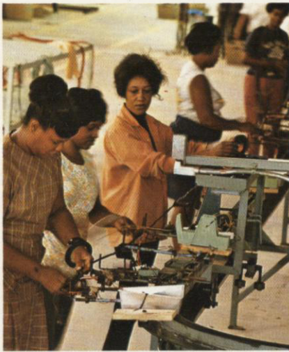
ITT Thompson Industries' new plant in Fayette, Mississippi produces electric wiring assemblies for automobiles.
