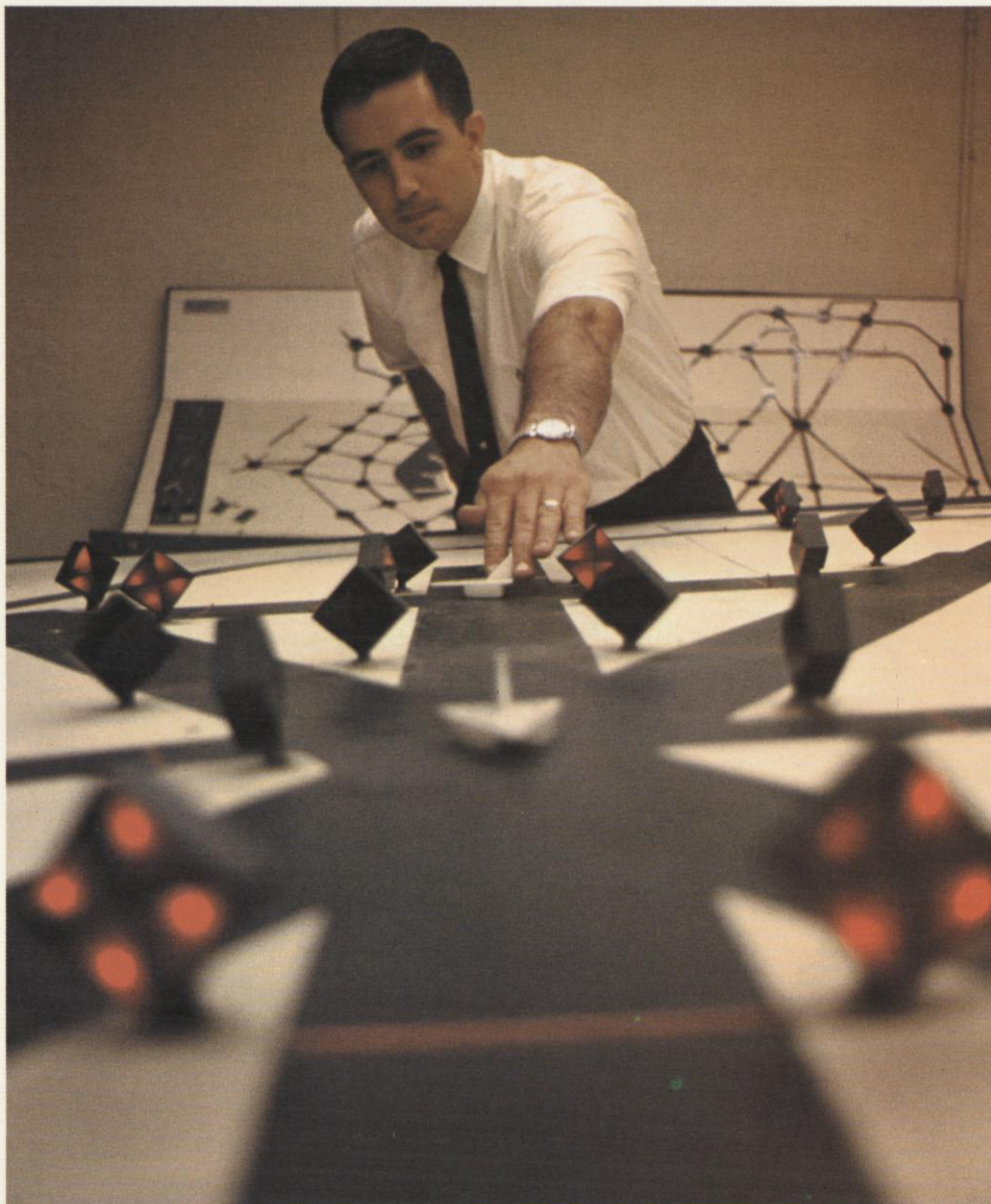
The ARROW (Airport Routing and Right of Way) system, developed at Bliss' Swarthmore Research Center, automatically routes aircraft on the ground, freeing the busy tower controllers.
