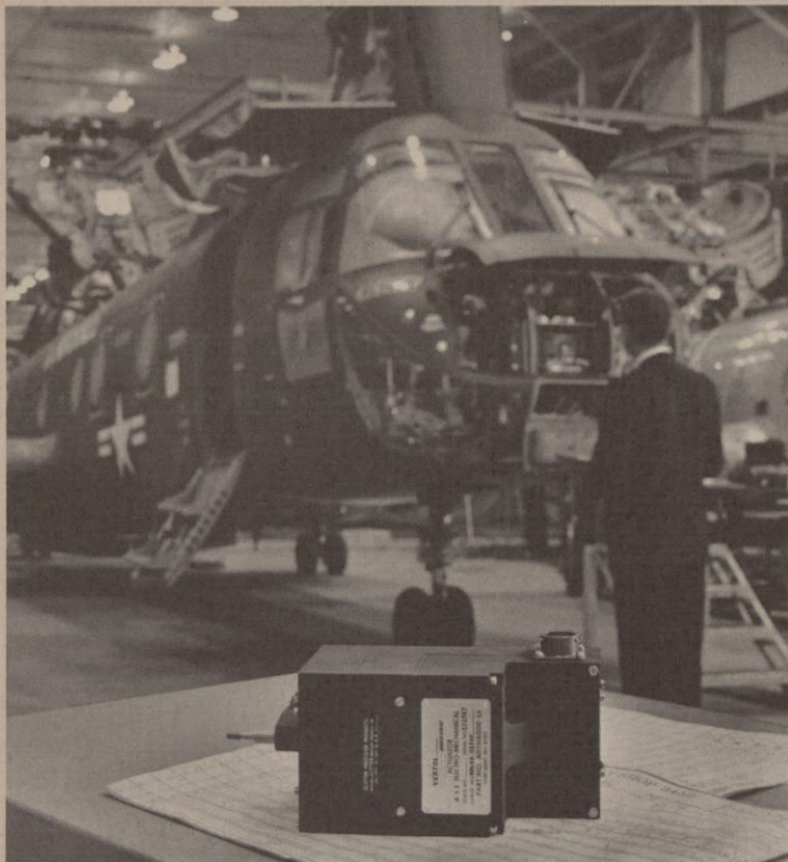
Clifton's automatic stabilization actuator (above) is used extensively in military helicopters such as this CH-46A Sea Knight.
