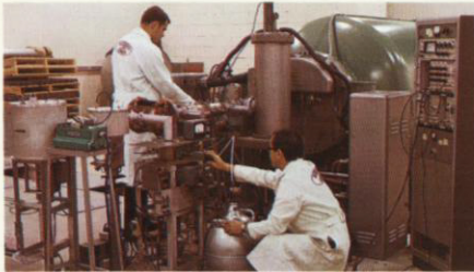
Technicians align an electron beam from the 3-million-volt Van de Graaff accelerator in the Nuclear Sciences Laboratory at the LTV Research Center. They are preparing to measure bremsstrahlung radiation from specimen spacecraft materials.
