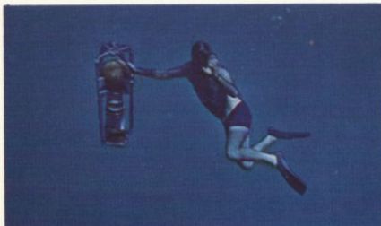
A recording sound velocimeter is lowered toward the ocean floor by a diver for the Research Center's Hawaiian Division.
