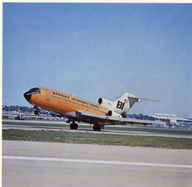
One of Braniff's 727-QC (Quick Change) transports can be switched from passenger service into a cargo plane in less than 30 minutes.
