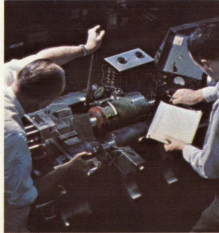
Experimental stress analysis test on a new Waterbury Farrel automatic machine, to be marketed in 1967.
