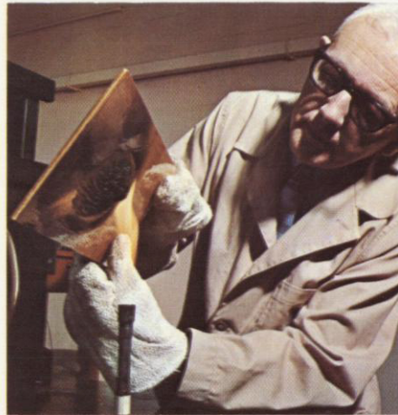
Spencer Kellogg research scientists have synthesized a urethane which foams and insulates, for use in fire retardant coatings.
