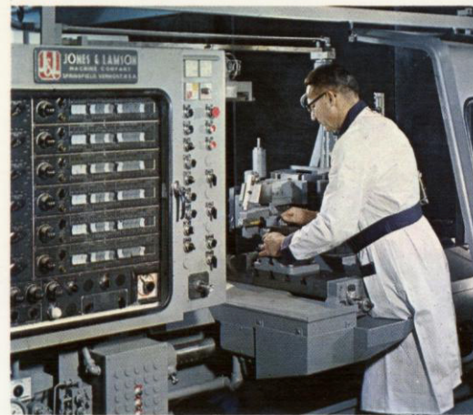
Jones & Lamson has developed a "new breed" of numerically-controlled turret lathes, in which dial settings program the machine through a solid state, built-in computer and positioning system.
