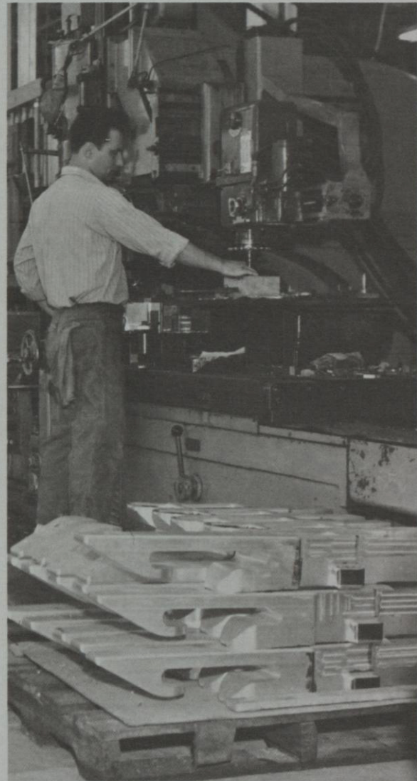
One of a battery of large contour milling machines is shown in Gulf & Western's new, modern plant in Pennsylvania. Here a craftsman is machining arresting hooks (right foreground) used with large nylon cable in the launching dolly assembly for catapulting aircraft.
