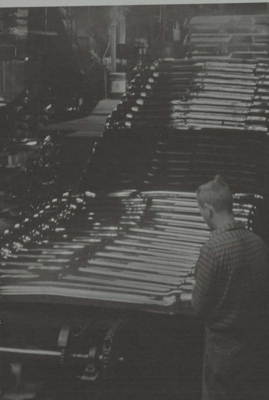
During each hour of operation, thousands of automotive parts or accessories come off this automatic continuous plater at Gulf & Western's Grand Rapids Brass Co. Moving counter-clockwise, the racked parts go through a series of steps in an electro-plating process where they are lowered into cleaning baths, plated with copper, then nickel and then chrome and finally moved out to a drying oven before being unracked.
