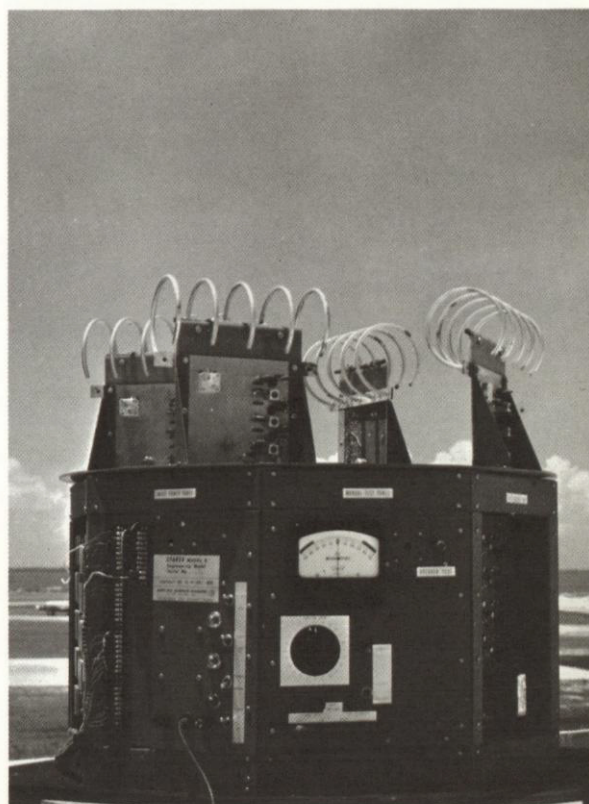
Photographed during installation at the Aerospace Instrumentation Laboratory, Patrick Air Force Base, Cape Kennedy, the SPARSA storm warning equipment is produced by Litton's Applied Science Division. The SPARSA system is designed to measure the strength and position of electromagnetic disturbances within a radius of 200 miles and to display data for detecting development of potentially dangerous storms on a closed circuit television triangulation console.
