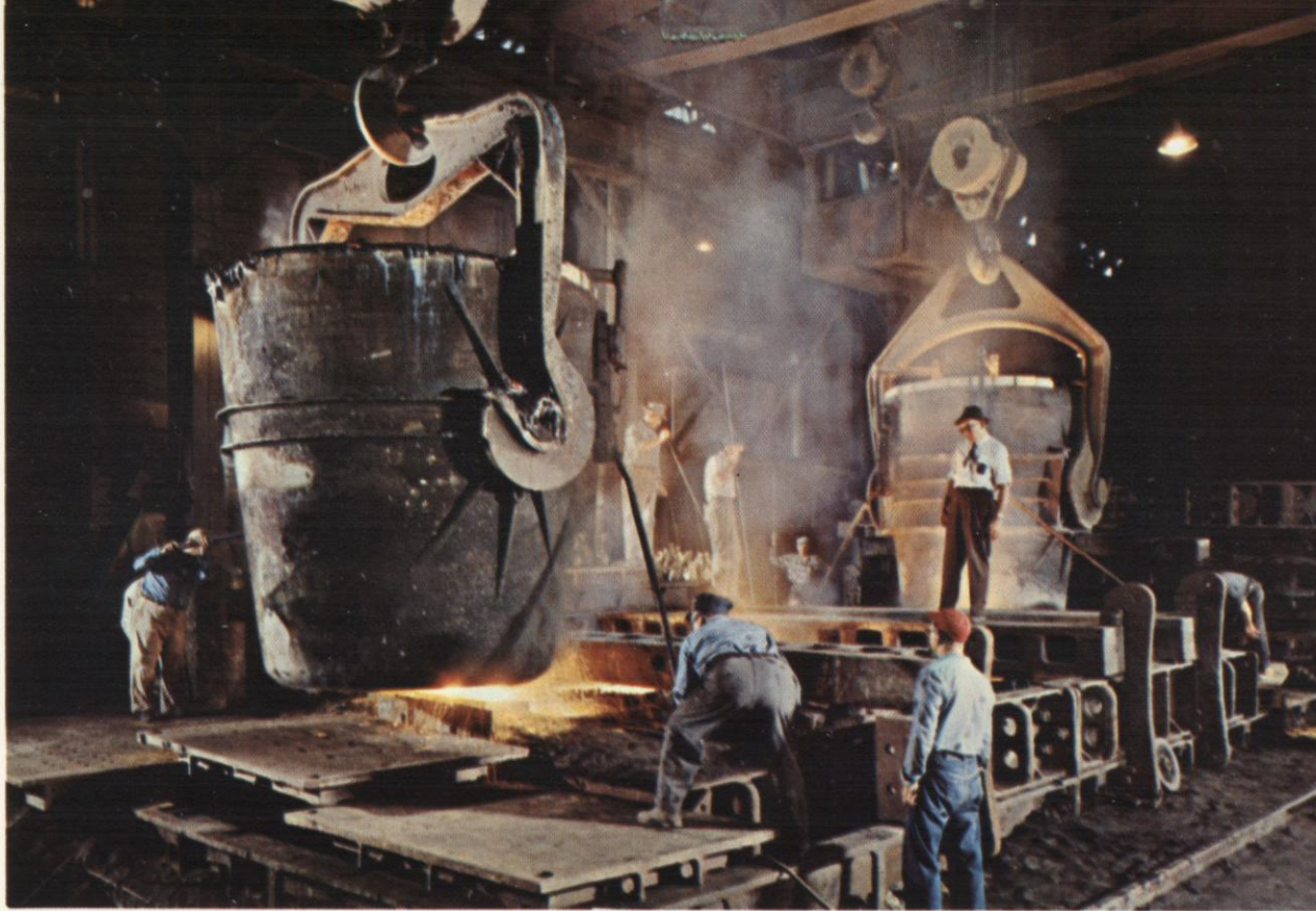
A steel casting weighing 100,000 pounds is poured in the plant of Pittsburgh Steel Foundry and Machine. The casting was used in an aluminum rolling mill designed and built by this Textron division.
