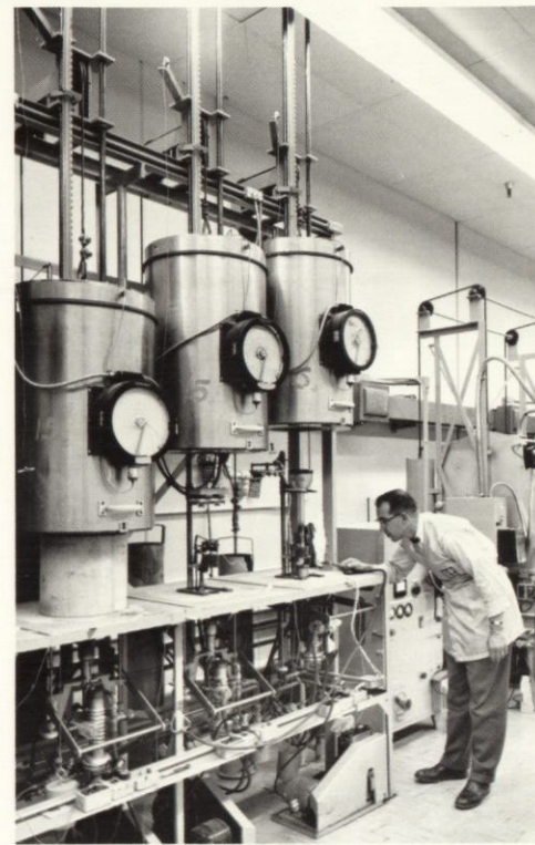
The Guidance and Control Systems division's new dust free area, among the finest in the world, makes it possible to increase substantially gyroscope production.
