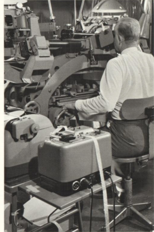
Four-color gravure press is among the unusual printing equipment in service at Eureka Specialty Printing division, Scranton, Pa.
