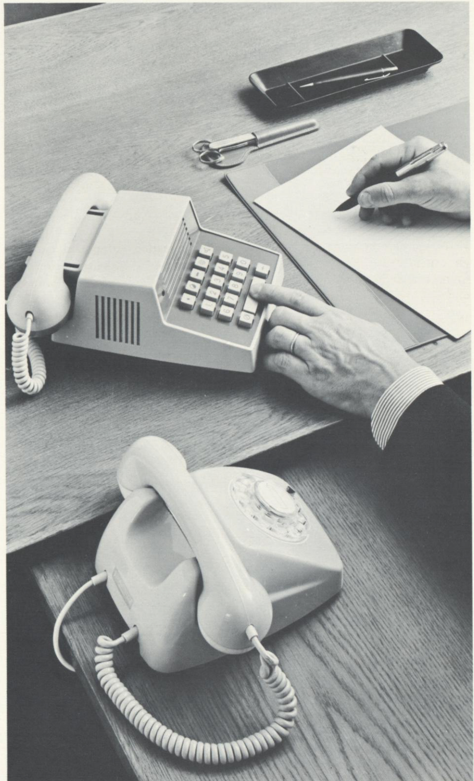
Manufactured by our Swedish company in its Solna plant, and marketed under the ITT Standard brand, the new intercommunication system pictured here features pushbutton call, hands-free operation, and direct selection. Sets are plug-and-jack connected for complete flexibility of movement.
