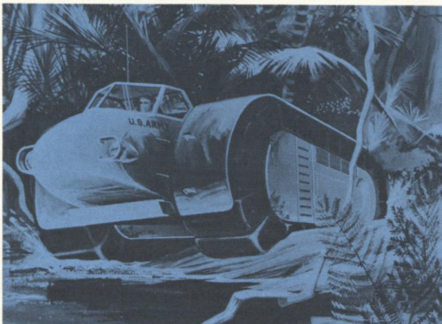
PAT , another newly-designed military vehicle, employs inflated rubber tracks to roll across obstacles deemed impassable .
