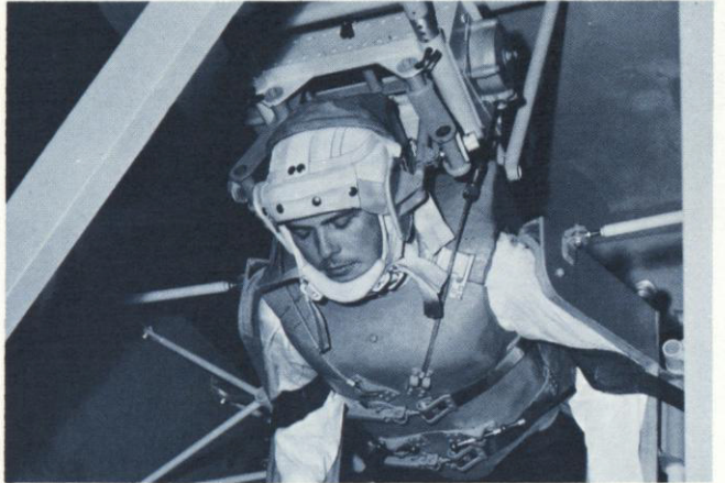
Company-designed astronaut restraint and protection system allows manual control during emergency hard-impact landings.
