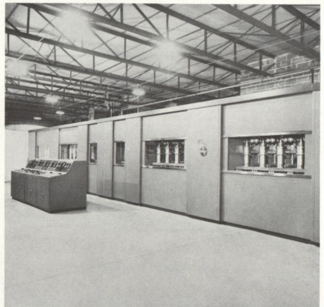
U.S. Information Agency utilizes LTV 1-million-watt shortwave transmitters to blanket world with Voice of America programs.
