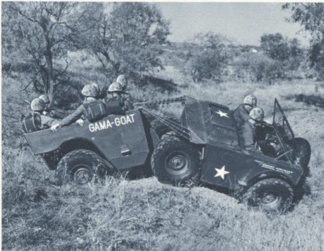
Gama Goat , designed to cope with rough terrain, demonstrates its ability to carry troops and supplies almost anywhere.
