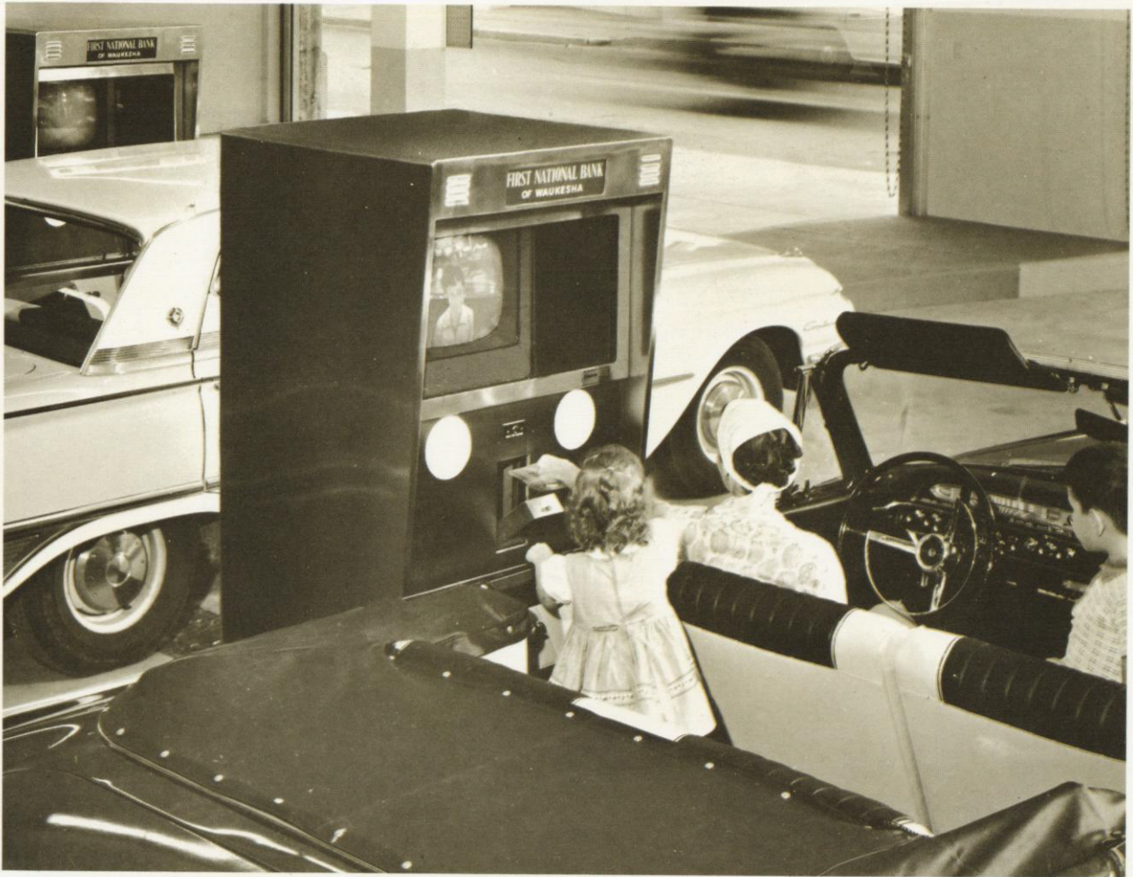
The country's first "Autobanker" system, a modern drive-in facility designed by the Mosler Safe Company and engineered by ITT, was installed in 1961 at the First National Bank in Waukesha, Wisconsin. The facility enables customers to transact most of their banking business from the front seats of their automobiles.
