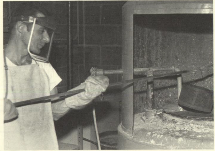
One of the advanced methods used by The Klock Corporation in the thermal processing of metals for spacecraft is the nitriding of stainless steels. This process permits the engineer to select and harden a specific area of the metal surface.
