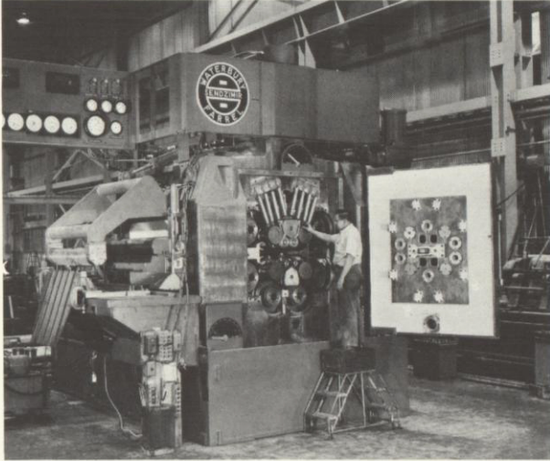
Sendzimir mill built at Waterbury Farrel plant for cold rolling of very thin tinplate.
