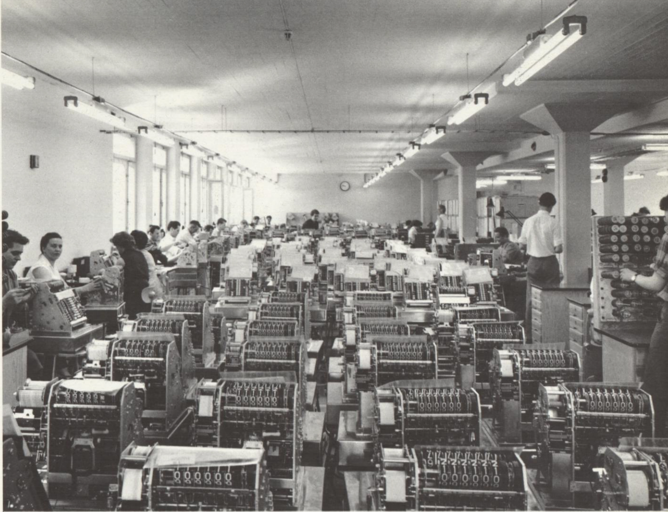
INSPECTION OF CASH REGISTERS REQUIRES TESTING OF OPERATING CHARACTERISTICS AT THE PLANT OF SVENSKA DATAREGISTER, A.B., IN STOCKHOLM, SWEDEN
