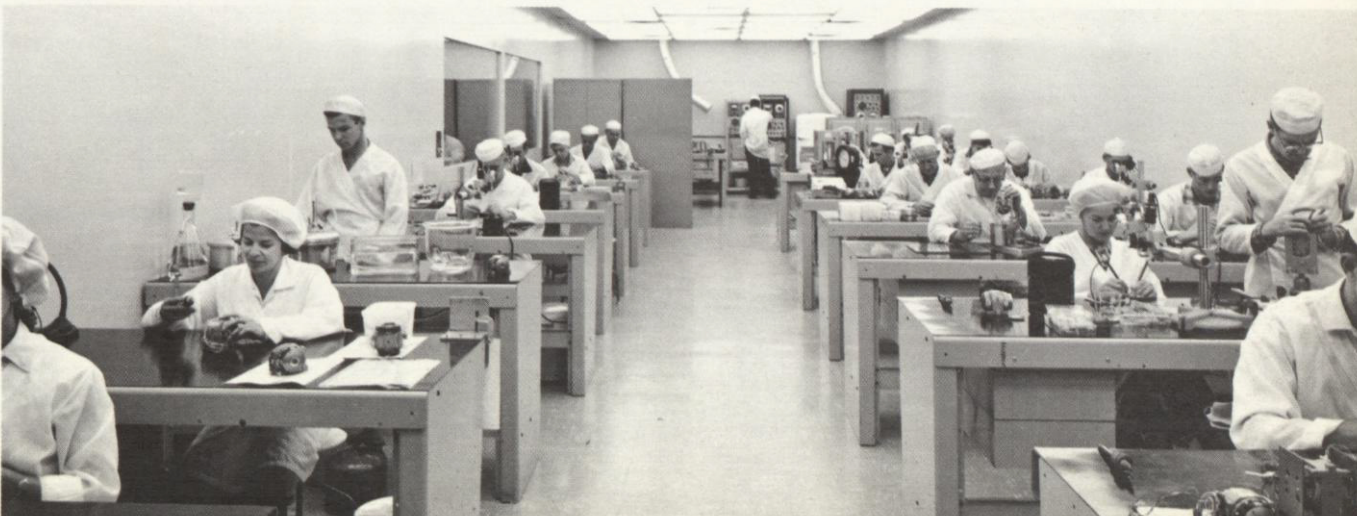
HIGH PRECISION GYROS MUST BE ASSEMBLED IN DUST-FREE, HUMIDITY AND TEMPERATURE-CONTROLLED ROOMS LIKE THIS IN THE PLANT AT BEVERLY HILLS, CALIFORNIA
