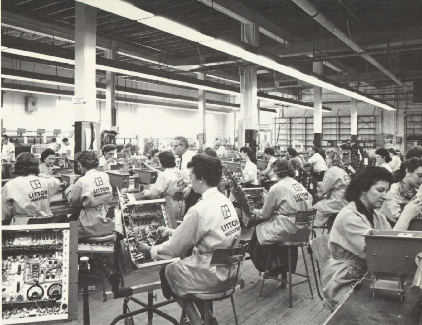
MONITORS FOR AVIATION INSTRUMENT LANDING SYSTEMS ARE ASSEMBLED ON THESE PRODUCTION LINES OF THE MARYLAND DIVISION IN COLLEGE PARK, MARYLAND
