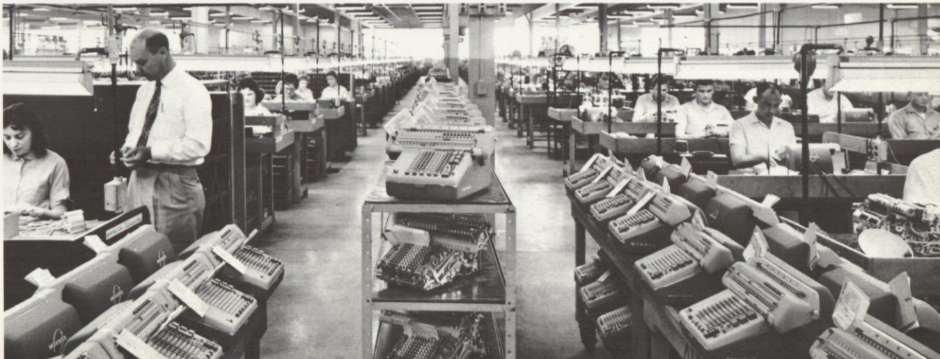
SCORES OF THE LATEST MODEL MONROE BUSINESS MACHINES ARE SHOWN ON THE FINAL ASSEMBLY LINE AT THE MONROE DIVISION'S PLANT IN BRISTOL, VIRGINIA
