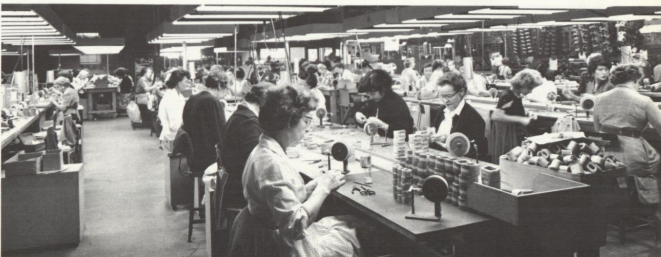
INSPECTION AND CHECK-OUT OF COIL WINDINGS FOR TRANSFORMERS IS DONE ON THIS LINE AT THE TRIAD CORPORATION DIVISION IN VENICE, CALIFORNIA
