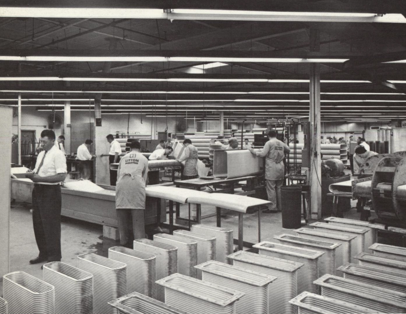
ALL-ALUMINUM WAVEGUIDES OF VARIOUS SIZES FOR RADAR SYSTEMS ARE SHOWN IN THE FINAL ASSEMBLY DEPARTMENT AT THE PLANT OF AIRTRON AT LINDEN, N.J.
