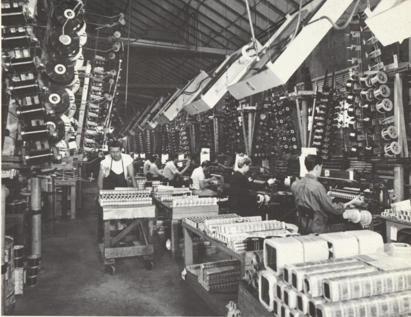
COIL WINDING MACHINES SELF-DESIGNED BY THE TRIAD CORPORATION IN VENICE, CALIFORNIA ARE USED TO PRODUCE A WIDE VARIETY OF HIGH QUALITY TRANSFORMERS
