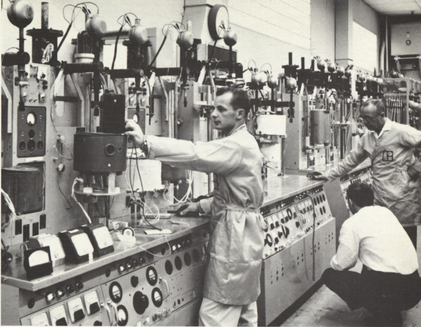
TECHNICIANS SUPERVISE OPERATIONS AT THE TRAVELING WAVE TUBE EXHAUST STATIONS AT THE SAN CARLOS, CALIFORNIA PLANT OF THE ELECTRON TUBE DIVISION
