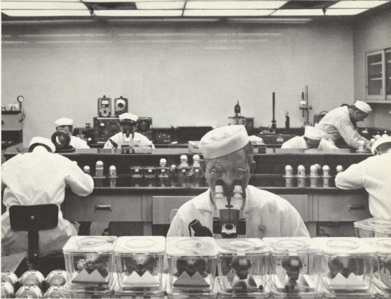
STANDARDS OF GYRO BEARING ASSEMBLY ARE MEASURED IN MILLIONTHS OF AN INCH IN BEVERLY HILLS, CALIFORNIA. FINGERPRINT-THICK ALIGNMENTS ARE NECESSARY
