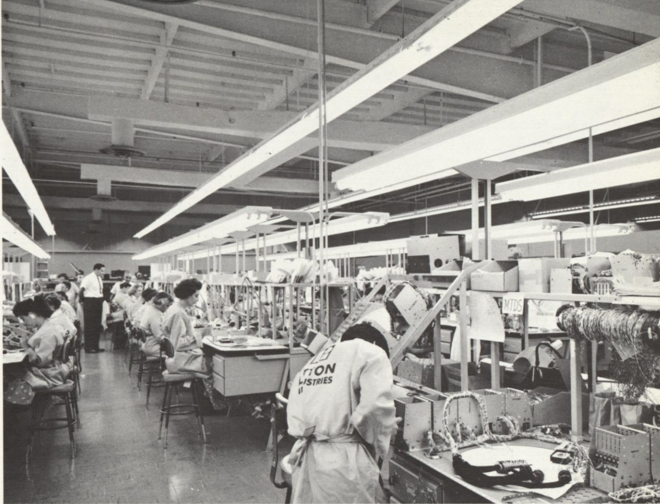
SKILLED ASSEMBLY IS REQUIRED FOR AN AIRBORNE DATA SYSTEM WITH 1,000 CIRCUIT BOARDS AND 55,000 TRANSISTORS AT THE CANOGA PARK, CALIFORNIA PLANT
