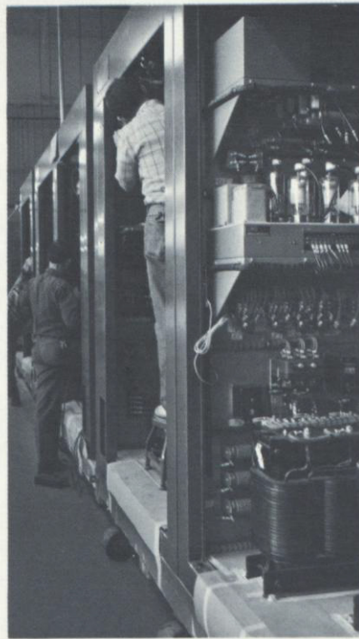
High-power amplifiers to drive electrodynamic vibrators manufactured by Ling Electronics.
