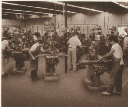
This interior picture of the Mal Tool plant shows a portion of the 42 milling machines which are used in the production of precision parts.
