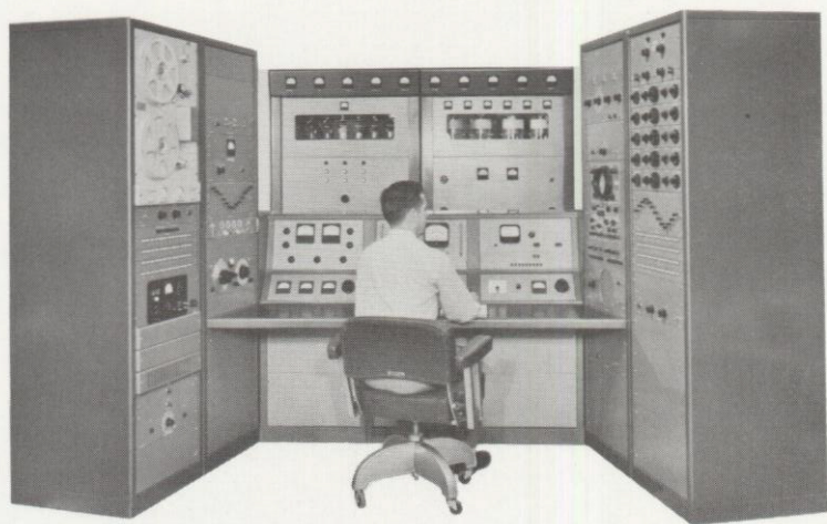
Equalizer-Analyzer Control and High Power System for Vibration Testing
