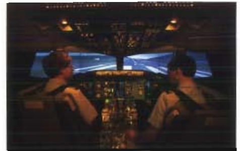
Certificated at Level "D", the highest of FAA-defined simulation standards, this Boeing 757 flight simulator serves the pilots of Spain's Iberia Airlines at SENASA's Madrid training center.
