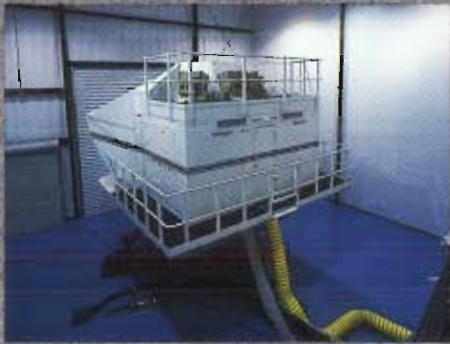
Advancing simulator technology has resulted in significant progress in the FAA-approved replacement of in-flight training with simulator-based training. The two Bell 412/212 helicopter simulators (above: the Bell 212) delivered in 1992 and 93 to the Company's Forth Worth training center, have demonstrated this. The FAA's approval now allows customer pilots to achieve certain qualifications for the first time without an in-flight aircraft check ride.
