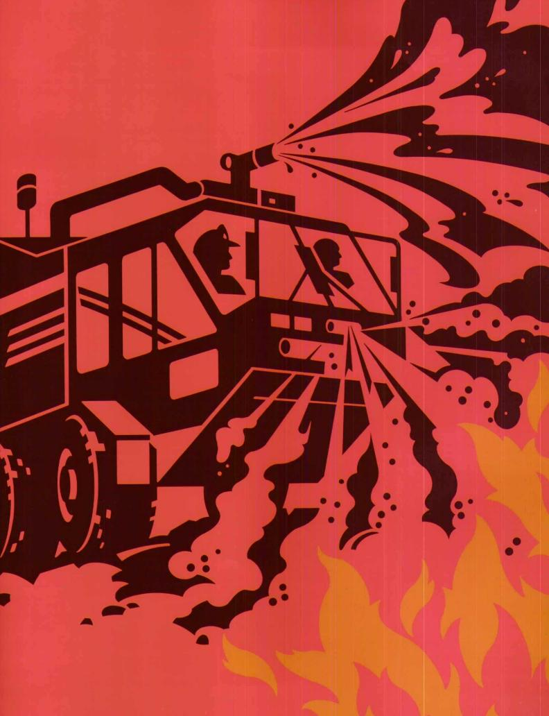
The front four wheels of the Crash Fire Rescue vehicle all turn to steer the vehicle, giving it great agility and positive steering response in cross country travel. These four wheels, as well as the rear four are all independently suspended and power driven.
