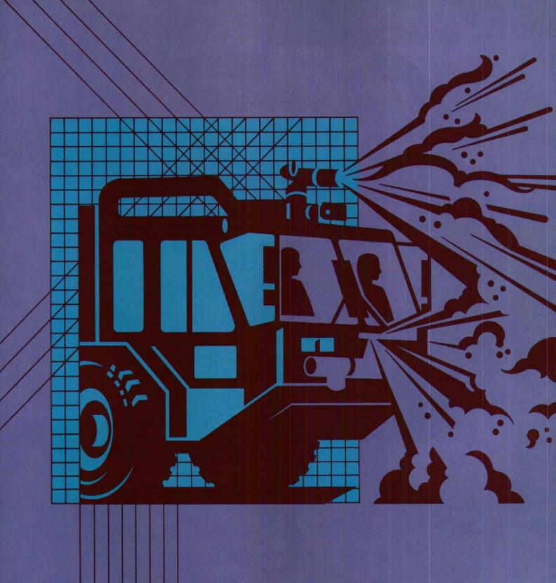
Power for the CFR's state-ofthe-art fire fighting system is provided by the vehicle's 575 horsepower turbocharged diesel engine, which permits it to discharge up to 1500 gallons of fire fighting agent per minute. The vehicle can maneuver while pumping, an important capability in producing the maximum fire quenching effect at the crash site.
