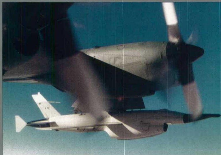
The AQM34M RPV, suspended beneath a wing prior to launch.
