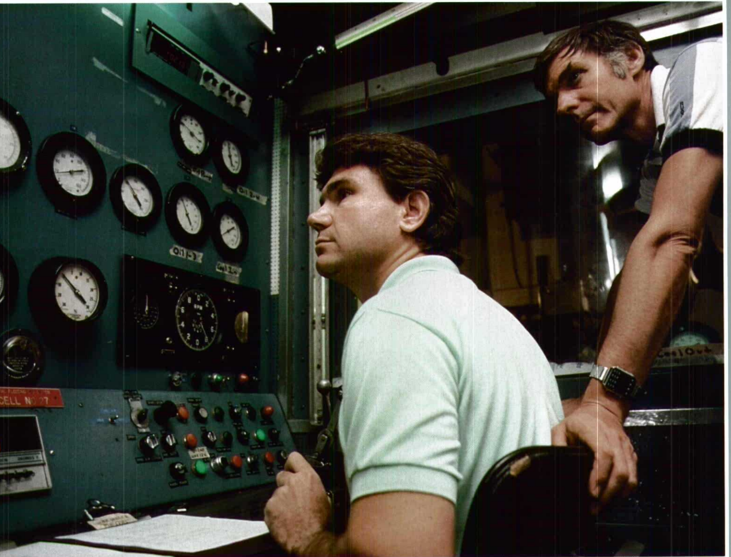
Voyager pilot Dick Rutan (right) made many visits to the Teledyne Continental plant in Mobile, Alabama where the Voyager engines were made. Here with a technician he checks out performance while the experimental liquid cooled engine runs in a test chamber.
