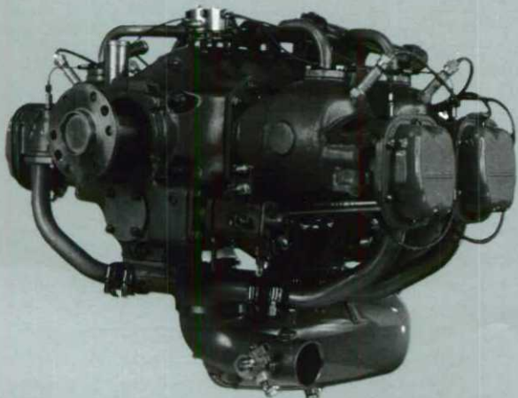
Model: Teledyne Continental Voyager-200 Production: Experimental Cooling: Liquid Horsepower: 110 Voyager: Main Engine, Rear, Pusher Running Time: 216 Hours
