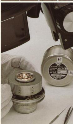
Teledyne's unique strapdown gyroscopes are assembled and adjusted under clean-room conditions. Each gyroscope provides information on two axes of motion.
