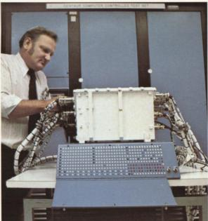
Computers are so fast it takes another computer to check them out. The full-scale blue computer controlled test set in the background is putting the white DCU through its paces and monitoring the results.
