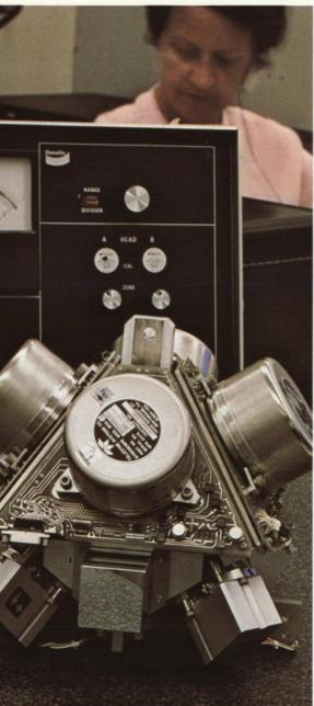
Teledyne's new inertial platform for the Interim Upper Stage of the Space Shuttle features four strapdown gyros, each giving two axes of reference for a total of eight where only three axes of reference data are required. This complete redundancy assures utmost reliability.
