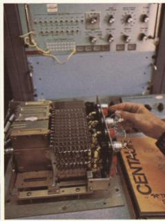
Teledyne also produces three multiplexer units, such as the one shown here under test, for each Centaur launch guidance system. These units gather data from sensors on the launch vehicle, format it and provide it to the computer as needed.
