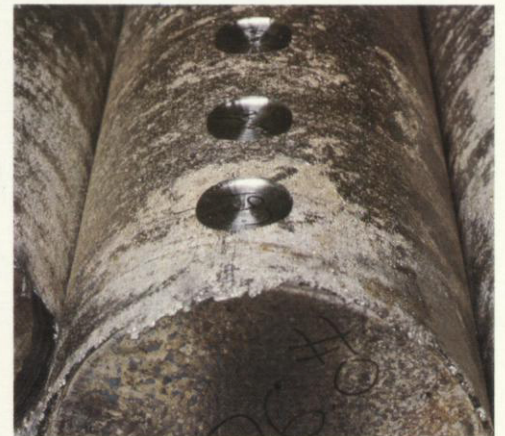
Zirconium tube blanks ready for conversion to finished tubing.
