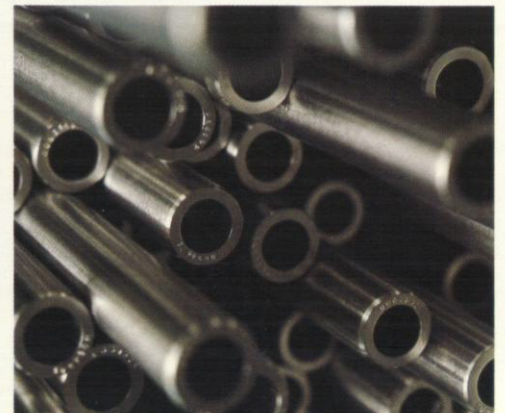
Zirconium tube blanks ready for conversion to finished tubing.
