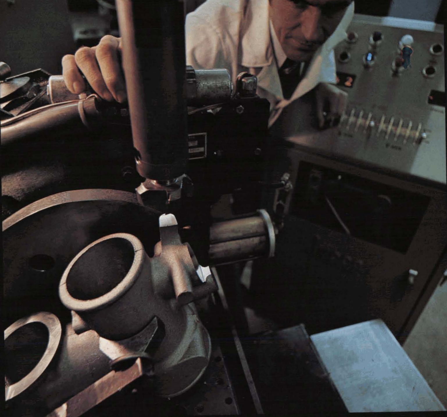
Right: Another type of automatic special purpose machine is used to bore the wrist pin hole and drill oil smoke holes in a Tiara engine piston.
