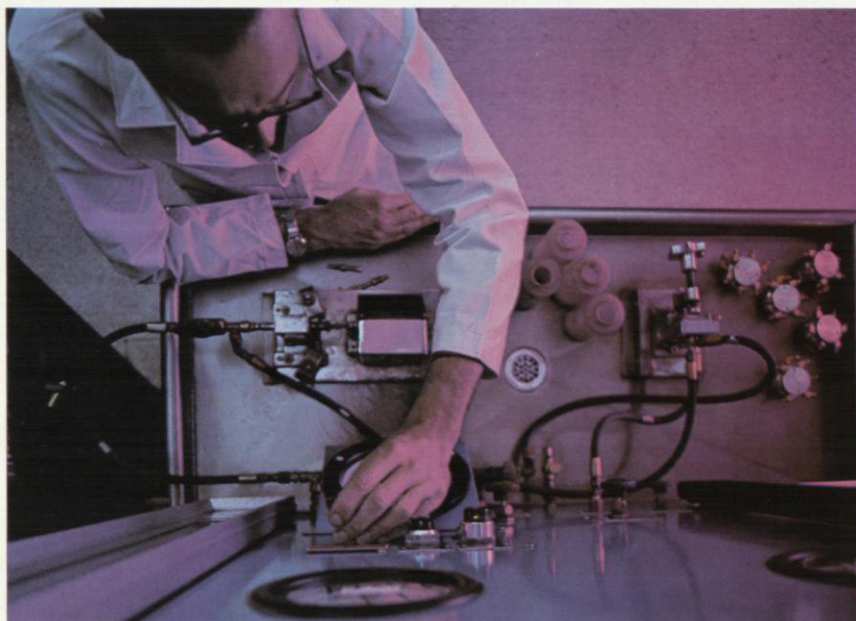
Top Left: Fuel metering accuracy in fuel injection systems is critical to engine performance. A series of test stands such as this one are used to calibrate fuel injection systems and components for uniform output.
