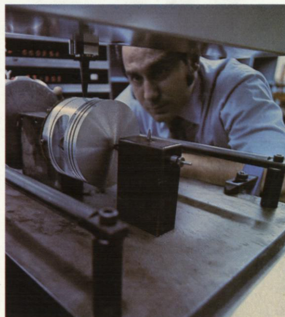
Top Left: Fuel metering accuracy in fuel injection systems is critical to engine performance. A series of test stands such as this one are used to calibrate fuel injection systems and components for uniform output.
