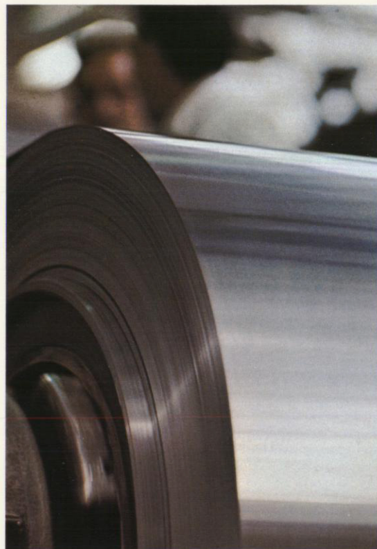
Stainless steel in the process of being rolled to a specified thickness is shown being recoiled at one end of the rolling mill. Stainless steel alloys of many types make up one of the most important classes of material rolled by Teledyne Rodney Metals.
