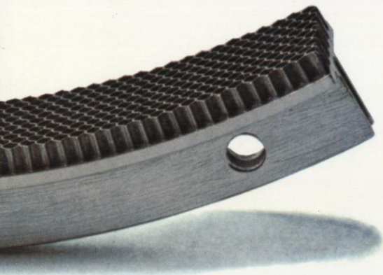
Effective gas seal between the rotating and stationary parts of high performance jet engines is provided by curved segments of honeycomb structure made of high temperature thin metal alloy.
