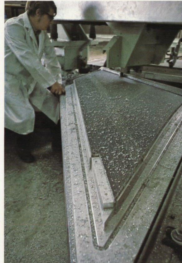
A special tape controlled machine tool designed and constructed by Teledyne Ryan Aeronautical automatically shapes an entire panel of aluminum honeycomb core to the exact contour of a wing airfoil. Tolerance is held to within 1/1000th of an inch.
