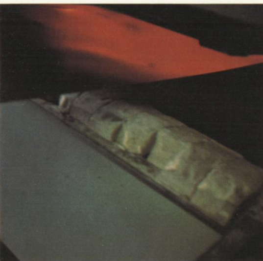
A strip of metal entering the annealing oven reflects the red glow of radiant heating elements that heat it to 2000°F. under controlled atmosphere to recrystallize its grain structure.
