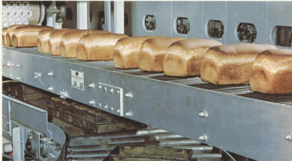
Specialty bread that has been proofed and baked by automated Teledyne Readco equipment is automatically moved to a Teledyne Readco bread cooler, prior to further processing.
