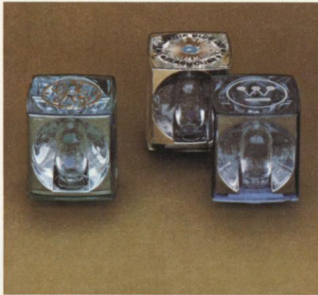
Zirconium, one of Teledyne's atomic age metals rolled to foil 8/10,000th of an inch thick, produces a brilliant flash of light when it burns in the oxygen-filled bulb of a flashcube. Hafnium, another Teledyne metal, is being introduced in new higher-output flashcubes.
