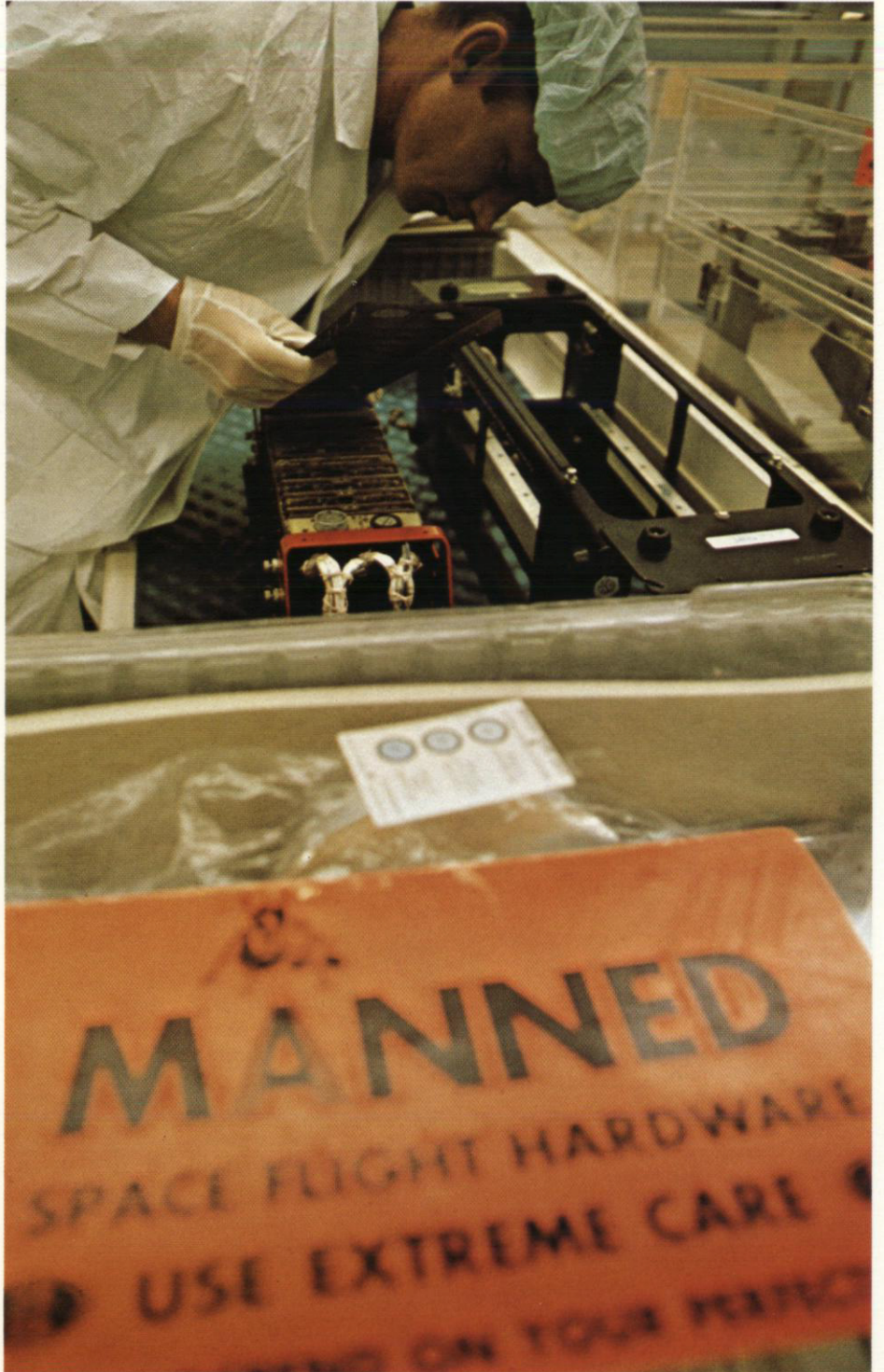
Completed electronic assembly of the Apollo Lunar Module landing radar is readied for final acceptance testing and shipment. Frequency trackers, signal data converters and power supply are packaged with the unit, which measures approximately 7 x 7 x 16 inches.
