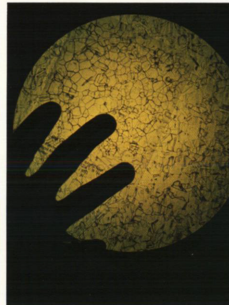
Grain-size determination of a superalloy sample at 100 times magnification is made on a metallographic microscope by comparison with an ASTM Standards chart. Metallographic inspection is a specification requirement of Teledyne Allvac superalloys to insure uniform distribution of particles and absence of contaminants.
