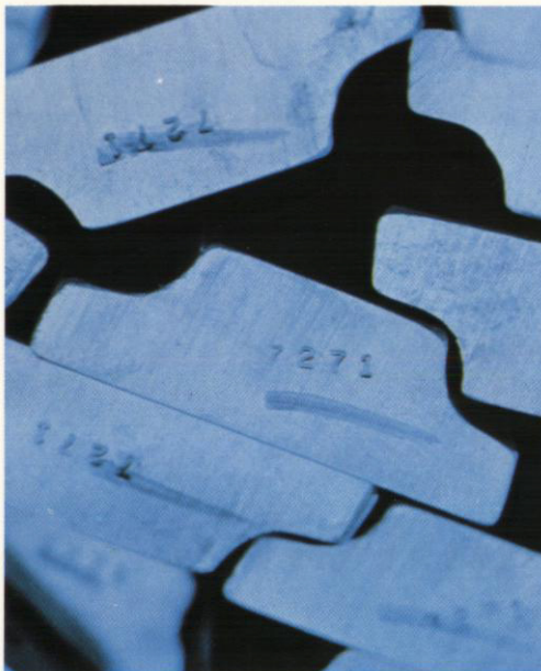
Metallurgical examination is made of superalloy materials at several stages in the production process, ranging from the raw ingot to the finished product. These macro slices for quality control inspection are cut from the ends of hot-rolled shapes intended for a jet engine application.
