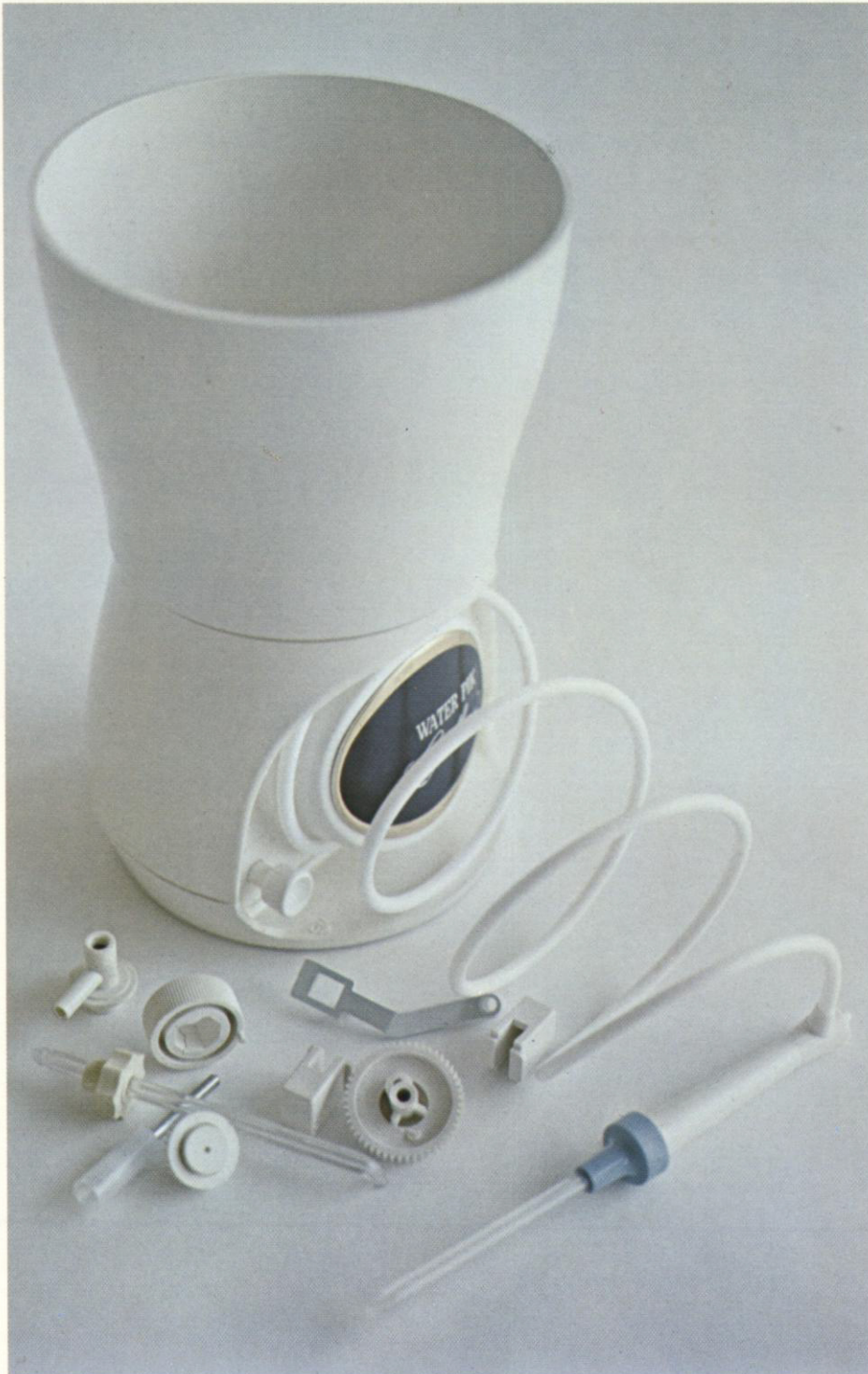
Eight different types of specialized engineering plastics are used in the fabrication of the Water Pik appliance. Each is chosen for specific physical properties such as hardness, flexibility, wear or impact resistance, or low coefficient of friction needed in some of the 80 parts of the device.
