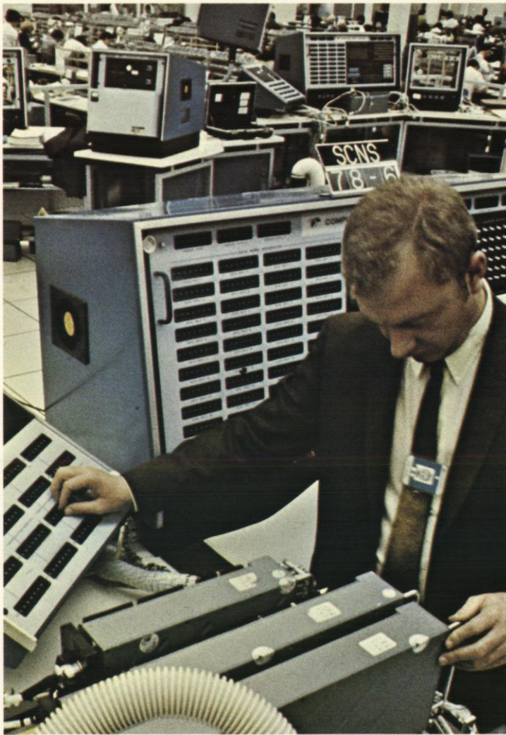
Final production acceptance testing of the three units comprising the CH-46 helicopter computer system is performed on semi-automatic test consoles.
