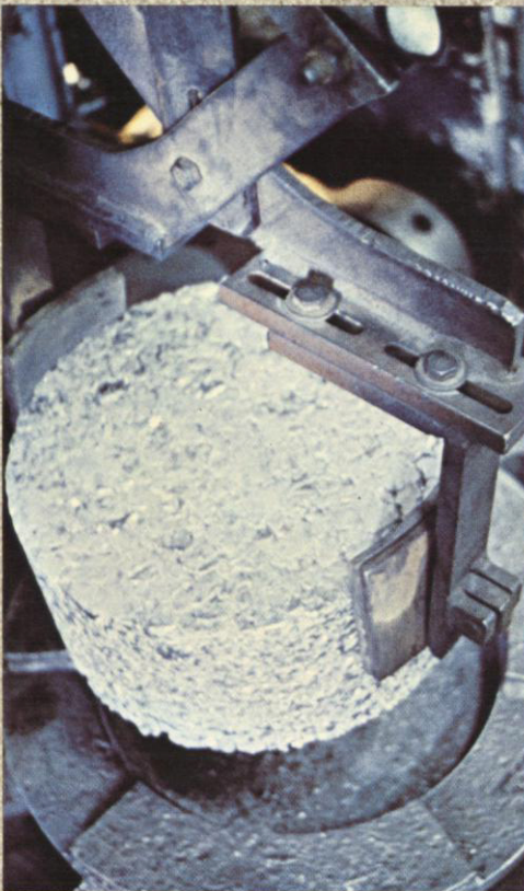
Crushed zirconium sponge is formed under high pressure into an 11-inch diameter slug for further processing.
