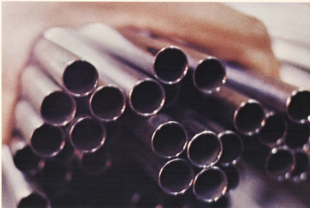
Reactor fuel is contained in zirconium tubes approximately one-half inch in diameter.
