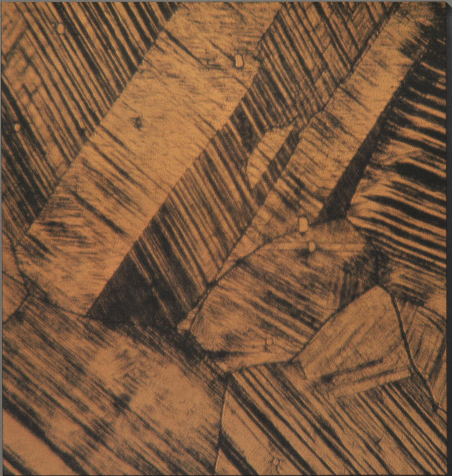
Microstructure of a superalloy is magnified 500 times after testing at high temperature and load for an extended period of time, in some cases up to several years. Information from tests aid metallurgical science to provide the key to advancements in such areas as aviation and space, where materials pace the realization of theory.
