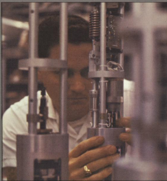
TOP: A Teledyne developed Apollo Lunar Surface Experiments Package that measures seismic motion will be left on the moon by astronauts as part of a program to determine the moon's composition and structure.
