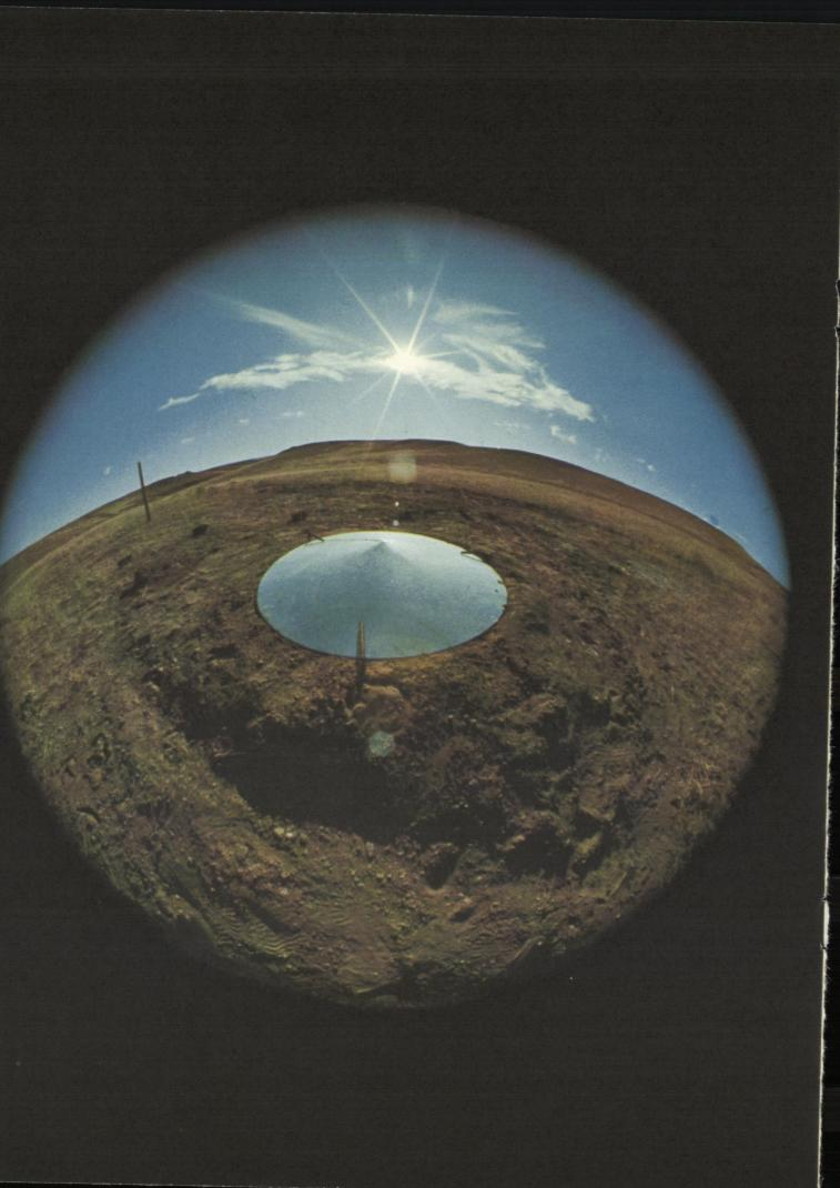
estled securely 200 feet below this conical metal cover in the open spaces of southeastern Montana is one of man's newest scientific tools—a highly sophisticated seismic ear sensitive to the faintest stirrings of the earth. This seismometer is just one of 525 similar instruments, deeply buried and carefully placed in a series of concentric patterns covering a 15,000 square mile area to form the Large Aperture Seismic Array, the most advanced seismological listening system ever assembled.
