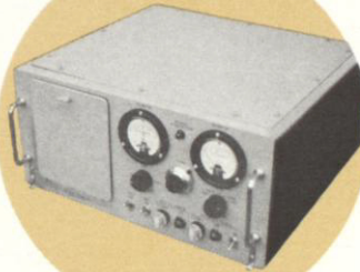
Phase-lock tracking receiver — used in tracking space vehicles.
