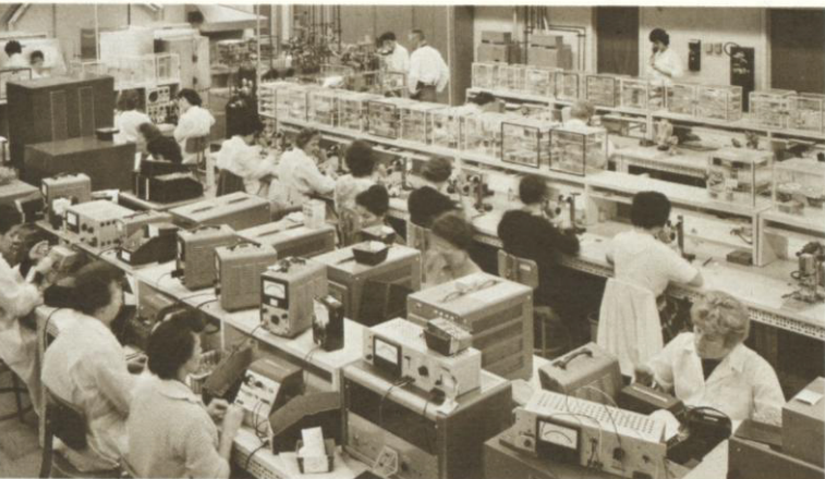
Semiconductor production area. Each unit is individually tested before and after final assembly.
