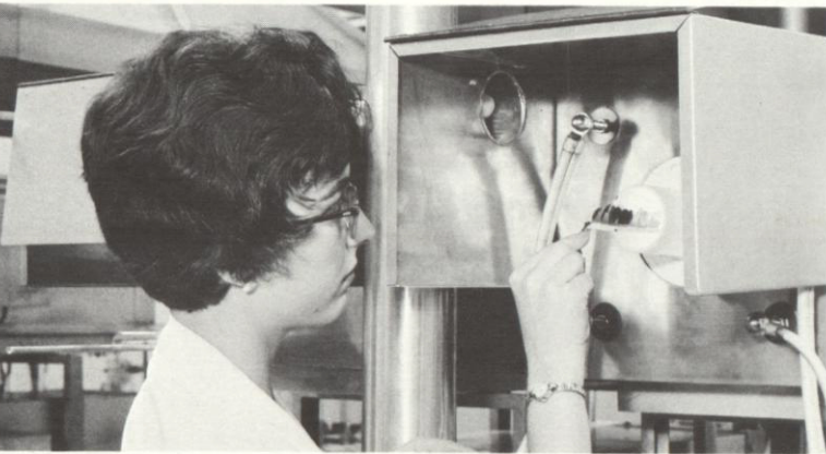
Removal of semiconductor wafers from diffusion furnace. This precision furnace, capable of extreme temperature control, is one of twenty-eight such units in use at Electron Devices Division.
