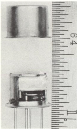
Subminiature electro-mechanical relay which provides reliable high-speed operation in a size heretofore unattainable.
