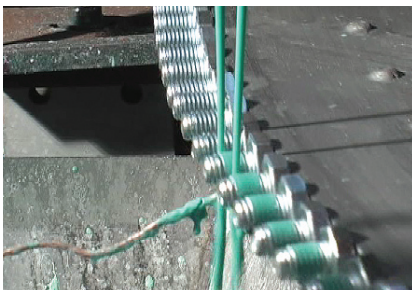
Nylok's patented coating processes are used to treat fastener threads.
