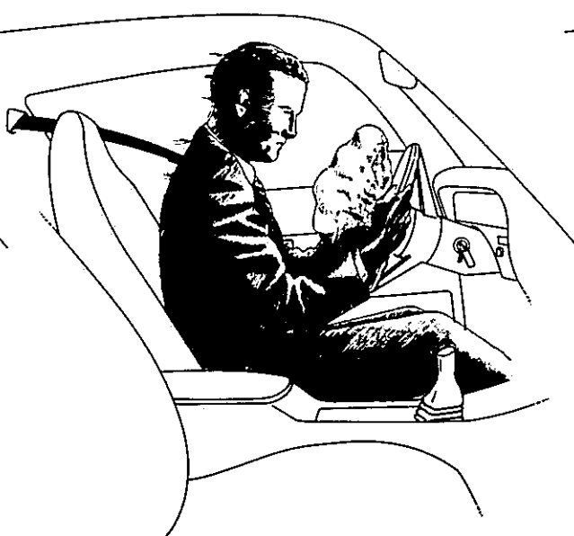
0.02 of a second — on impact, the car stops. Seat belt restrains the body but head keeps moving forward. Air bag fills to cushion driver.
