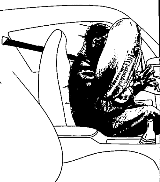
0.04 of a second — peak air bag inflation occurs to cushion driver, especially his head and face.
