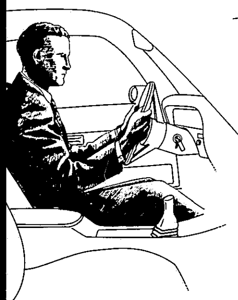
0.0 of a second — seat belt tightly fastened and air bag stored out of sight, ready to inflate in serious frontal crash.
