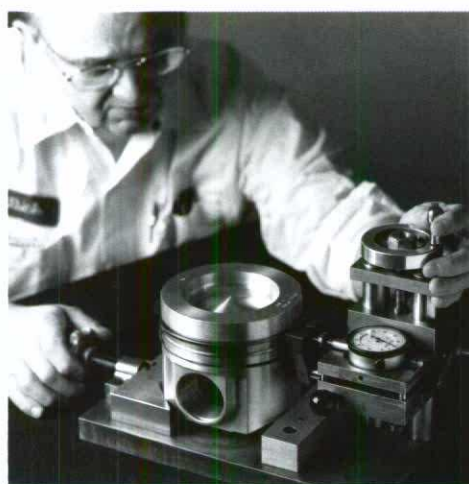
Piston ring rating: A precision instrument is used to determine heavy-duty diesel oil pass/fail results. One of the important criteria is the measurement of carbon deposits behind the piston rings.
