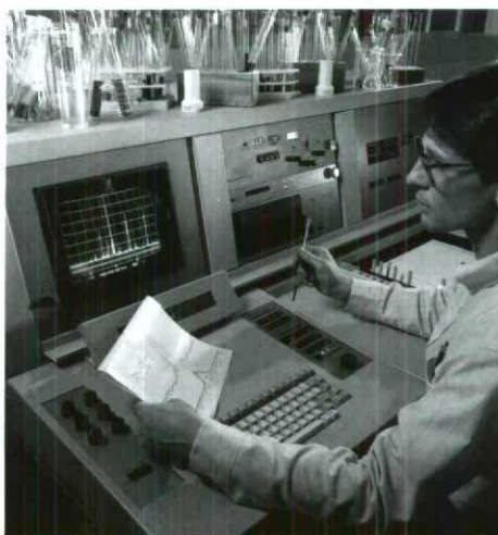
Advanced lubricant research: A nuclear magnetic resonance spectrometer at Lubrizol determines molecular structures of additive components to meet specific design requirements for lubricants.
