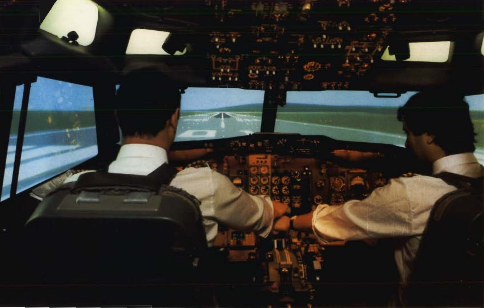
Flight simulator WIDE display system provides continuous field of view.
