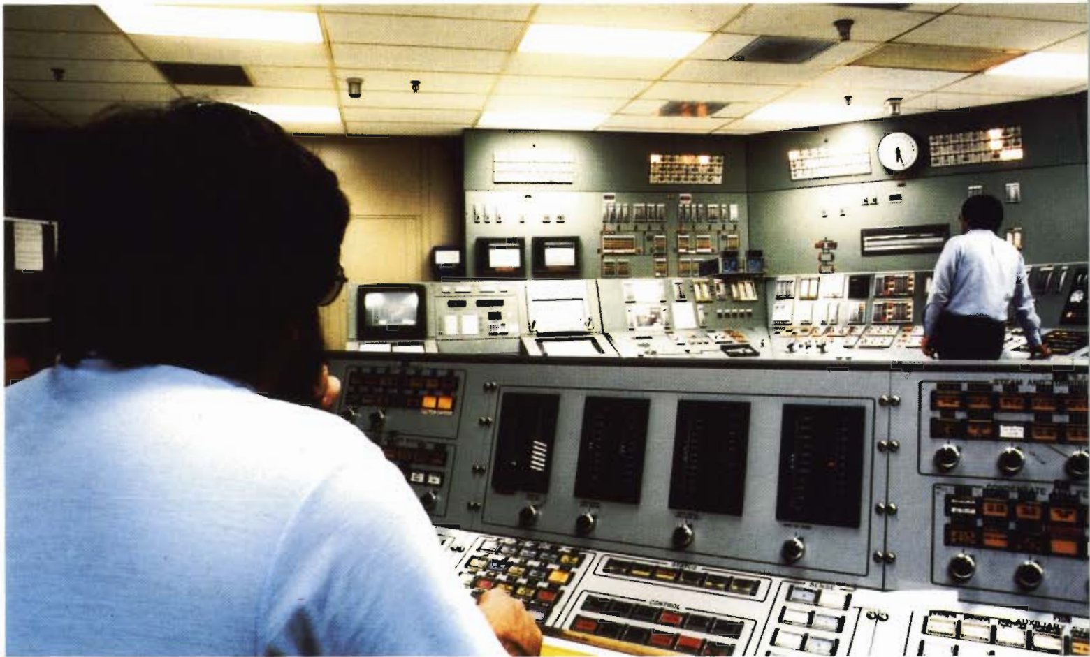
Full scale power plant simulator at Power Safety International. Simulator is an exact duplicate of Rancho Seco power plant, Sacramento, CA.
