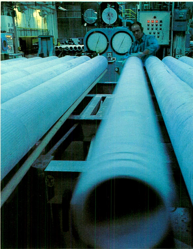
(Above:) Asbestos-cement pipe is dimensionally and visually inspected following beam testing for flexural strength.
