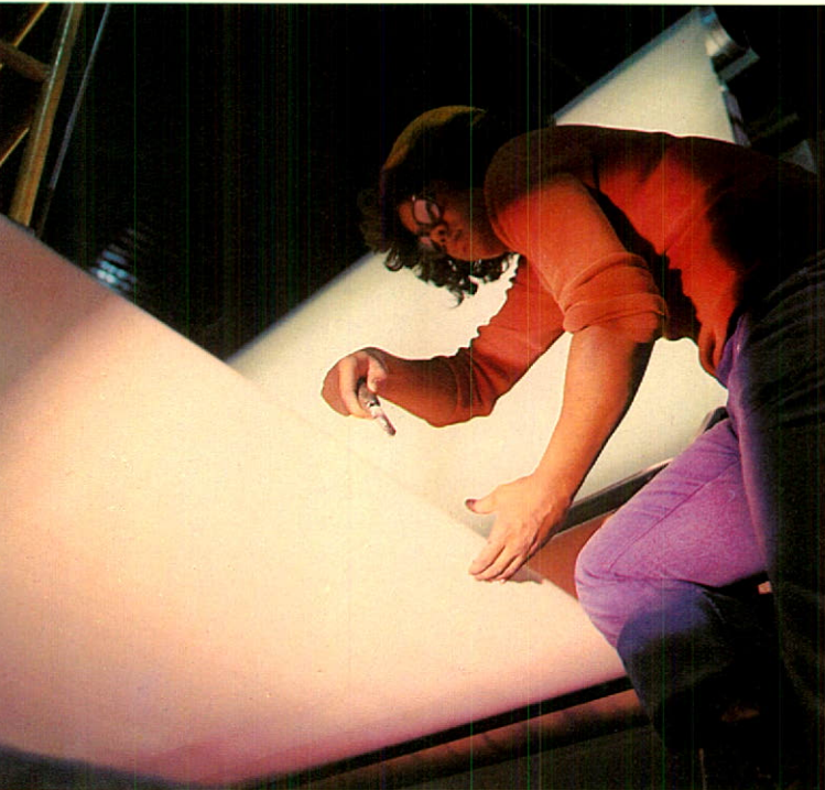
Thickness of fiber glass mat is carefully inspected as it emerges from a dryer. Demand for this specialized mat was accelerated in 1977 by the increased popularity of fiber glass roofing products in which it is used as a base.
