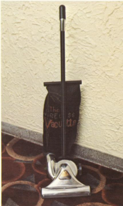
"The Wireless Vac-u-ette," an early model vacuum sweeper made about 1920 by the Scott & Fetzer Company. Non-electric, as it was moved over a rug, the side wheels turned a horizontal rotor which created an air suction. Dirt swept up by the roller brush in front was caught in the suction and propelled into the collection bag, which could be detached for emptying.
