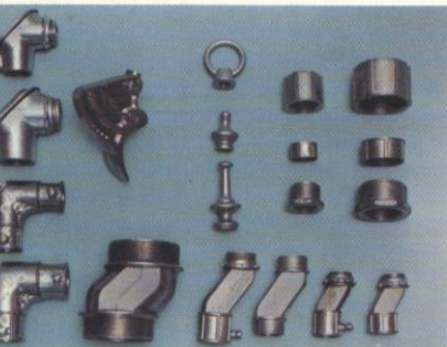
Finials for lamps, and typical die cast electrical conduit fittings made by the Halex Division
