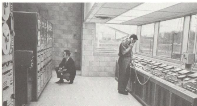
Operation of the road simulator is controlled remotely by instruments housed in this building.
