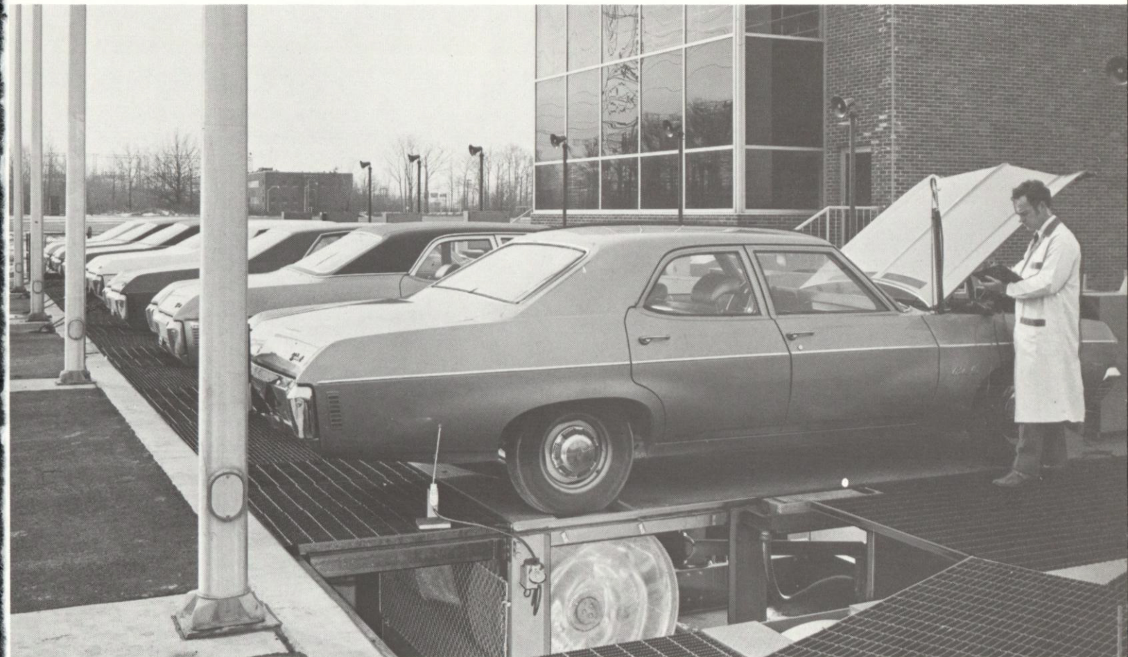
The road simulator, which is being expanded from four to eight lanes, is an effective tool for evaluating additive performance.
